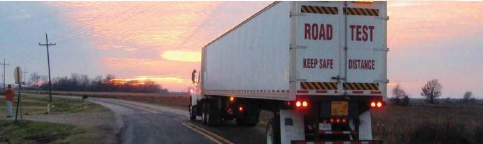
*The Rolling Wheel Deflectometer consists of a 55-ft. long semitrailer applying a standard 18,000-lb. load on a pavement structure by means of a regular dual-tire assembly over the rear single axle.*
